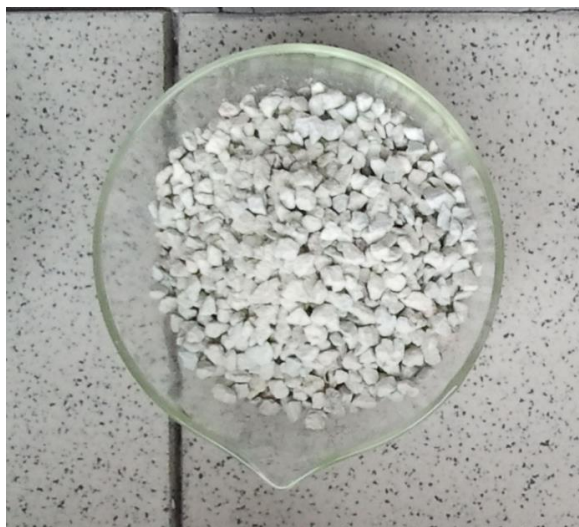
Figure 2. Zeolite with granulation coarse-grained 4,0-8,0 mm
