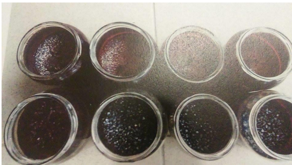
Figure 3. Probes of zeolites with manganese solution
