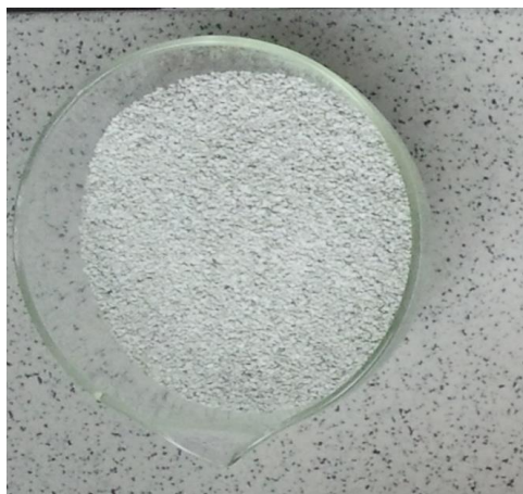
Figure 1. zeolite with granulation fine-grained 0,5-1,0 mm
